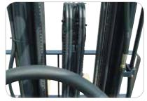
**Neatly arranged Hydraulic Hoses** Reduce clutter and provide better visibility.
